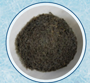
Cross-sectional area FIBALON ® ball (used)
